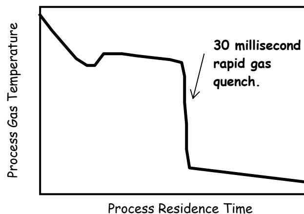
Figure 3. Schematic process gas temperature profile showing rapid gas quench.
