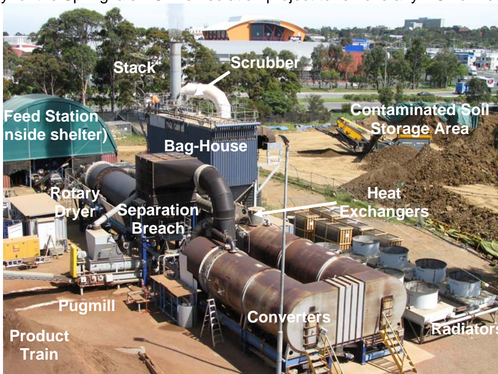
Figure 1: DFTD Process Overview
